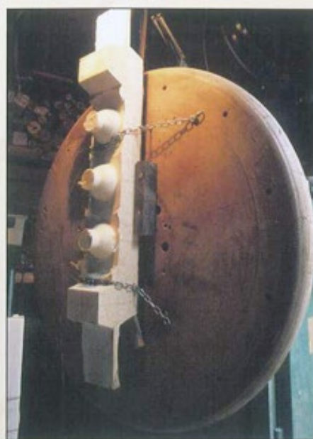
Starting with a long and thick chunk of wood, Mailland band saws a blank and mounts it outboard to turn five chucking spigots and vase bases; three of them have been completed.
