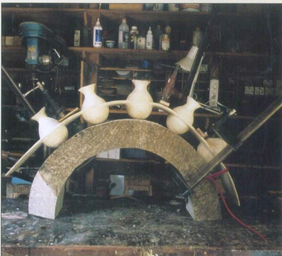
With the carving mostly completed, Mailland steams the wood and bends it over a curved form. After bending, he will carve the surface textures that enliven the completed piece.
